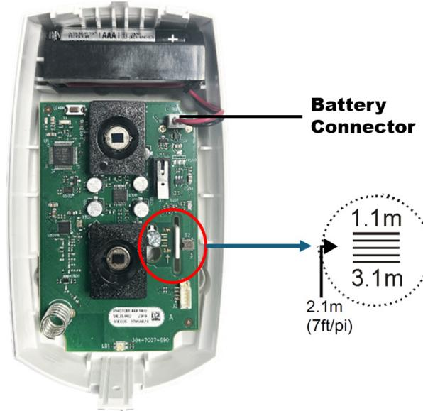
See the following figure for the beam dispersion at different height adjustments of the device board.
